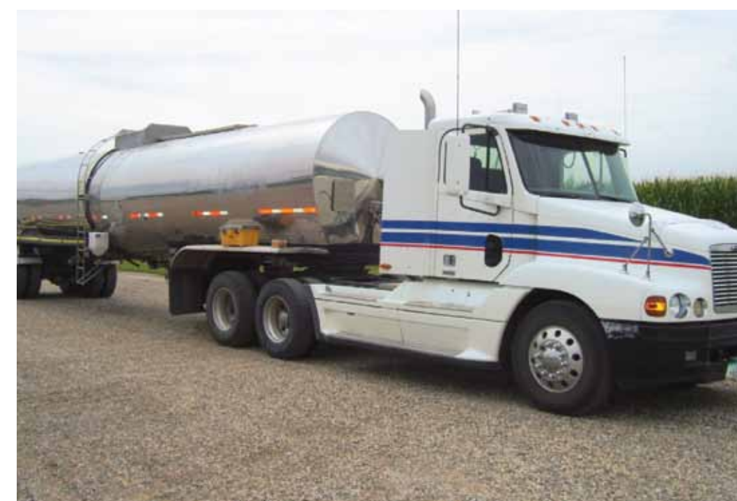
New stainless steel tanker used to mix and transport chemicals
