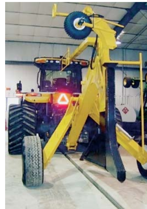
Tile plow with newly installed GPS.
